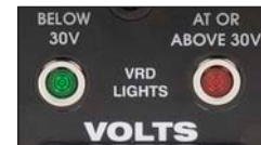
VRD® portion of nameplate with green light on.
